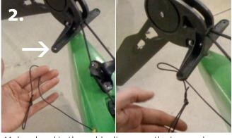
Make a bend in the rudder line as on the image above, and push the doubled up end through the hole in the rudder wing.
