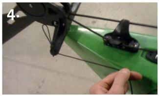
Pull the line tight so to fasten the loop. With this quick release knot, you can easily dismantle the rudder when transporting the kayak on land.
