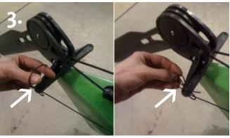
Pull the ready made loop at the end of the rudder line through the bend which was pulled through the hole.
