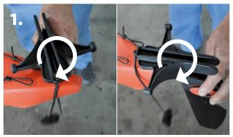
Install the rudder into the Rudder sleeve at the back of the kayak. Make sure the Rudder is turned as much toward the front as possible and turn it. In this position you should not be able to lift the rudder out of the rudder sleeve. If you can, you should turn it back into position and push down even further. (the rudder in this image is different, but the same method is applied)
