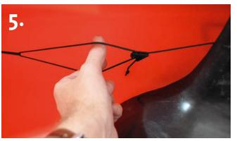
Tighten the rudderlines when sitting in the cockpit by adjusting the mini-line lockers. To tighten, pull the miniline locker towards the back. To loosen the lines do as on image above.
