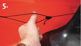
Tighten the rudderlines when sitting in the cockpit by adjusting the mini-line lockers. To tighten, pull the miniline locker towards the back. To loosen the lines do as on image above.
