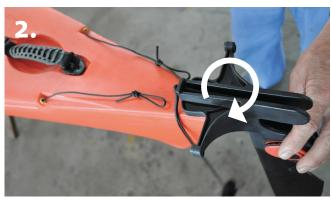
In this position you should not be able to lift the rudder out of the rudder sleeve. If you can, you should turn it back into position on image 1 and push down even further.
