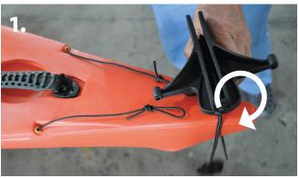
Install the rudder into the Rudder sleeve at the back of the kayak. Make sure the Rudder is turned as much toward the front as possible and turn it.
