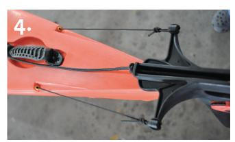
Pull the line tight so to fasten the loop in the groove. With this quick release knot, you can easily dismantle the rudder when transporting the kayak on land.
