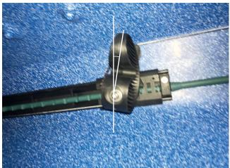
3. Tighten the line until the pedals are leaning slighty towards you as shown in the image above.
