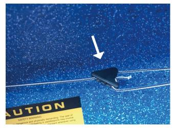
2. Tighten the rudder lines inside the cokpit using the miniline lockers on each side of the cockpit. To slacken the line, insert two fingers between the lines behind the mini-lin locker and pull them apart.
