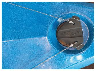
1. Put the ends of the rudder lines through the holes on each side of the rudder head at the back of the kayak. Turn the loops over the ends of the triangle shaped head to lock them into the grooves
