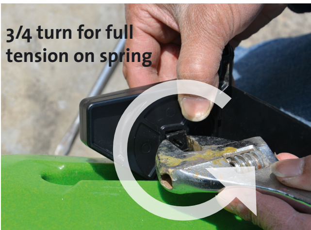
10. Push in the screw, but not all the way. Use the spanner tool to turn the screw a 3/4 quarter turn. You will need to push in your finger on the back side to prevent the screw to slide in.
