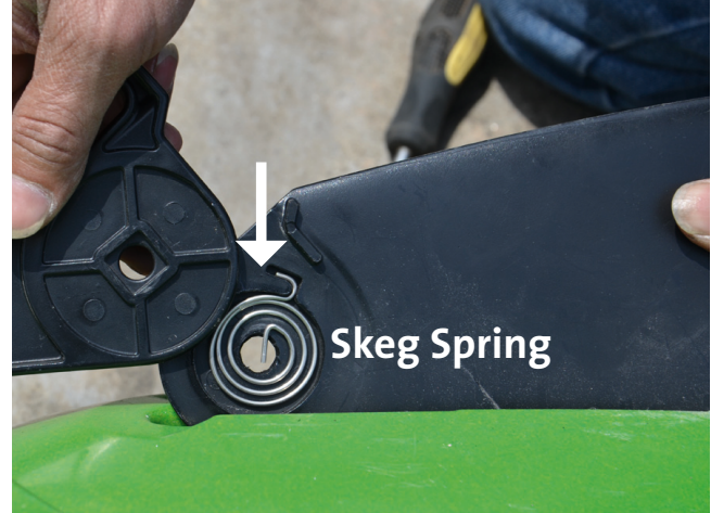
7. Slide out the skeg holder to reveal the spring. The spring in the image is a little deformed, but still operational. If the spring has been badly deformed or is broken, you need to replace it. Also check the plastic screw, which should be undamaged.
