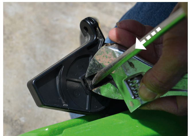
11. Turning the screw without the spring jumping out of the screw can be a bit tricky. You might need several tries to succeed. As the tension is high on the spring after the 3/4 turn has been completed you will need the screwdriver with flat head to push in the screw into its final position.
