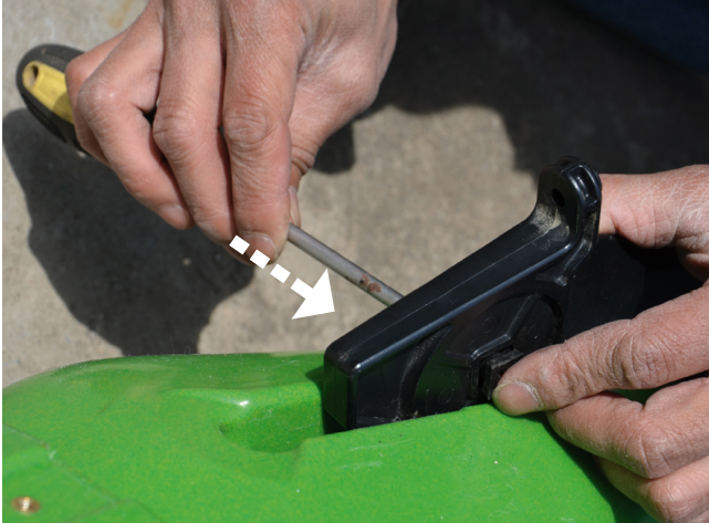
6. Push out the screw from the back using the phillips screw driver.
