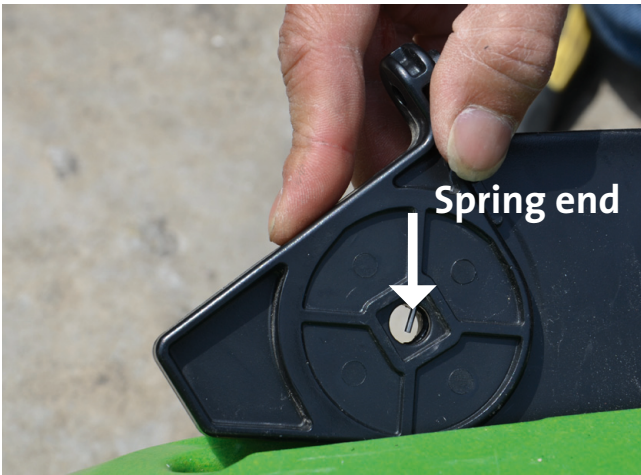
8. To assemble the skeg, slide on the skeg holder, make sure the spring end is in the middle of the opening.
