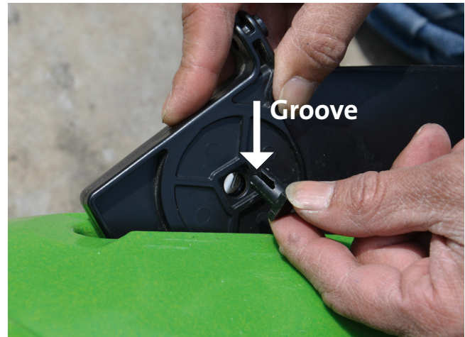
9. Put in the plastic screw, make sure the groove in the screw slides over the spring end.
