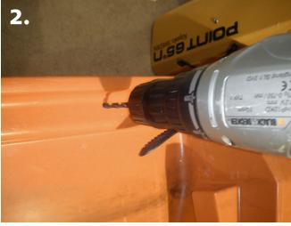
Use a 6mm drill to make the hole on each side of the cockpit.
