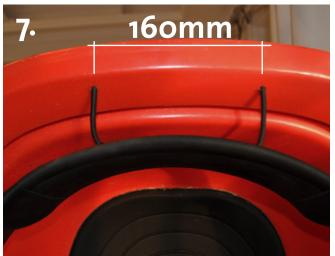
Drill 3/4" holes on the inside lip of the cockpit rim - DO NOT DRILL THROUGH THE OUTER RIM - or it will leak into the kayak through the holes!!! The holes should be equally wide apart from the center line of the kayak.
