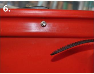
Fasten the nut with a washer between the nut and kayak. Don't pull too tight, but make sure the screw reaches the blue plastic locking thread on the nut.
