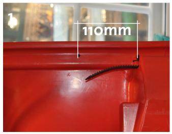
Measure the distance from the bulkhead on the side of the kayak as on the image above. Make sure the holw is centered. Do it again on the other side.
