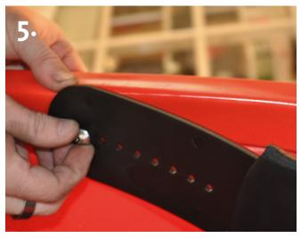
Push the screw from the inside of the cokpit into the plastic backbands outermost hole and though the drilled hole on the cockpit rim.
