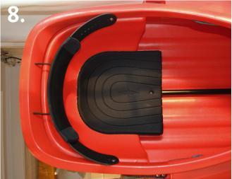
Pull the shock cord through the loops in the back of the back rest and through the holes in the cockpit. tie the ends together behind the backrest and cut off recess cord.
