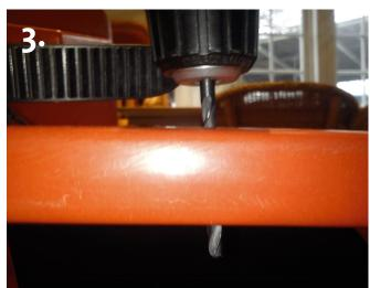
The drill should go though both layers of the cockpit
