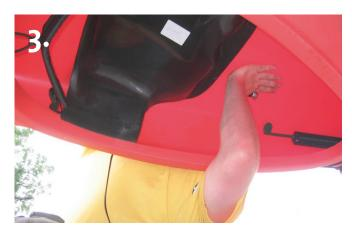
The plastic should never become too hot to touch or start melting (which is why we recommend a hair dryer as opposed to a heat gun usually used for scraping paint etc).
