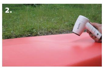
Start the repairing by heating up the dented area with the hair dryer, don't put it to close or you will get it too hot. When the plastic is heated you can start to apply pressure so that the plastic will get into its former shape. You will still have to use the dryer while doing it, so you might need some help from a friend.
