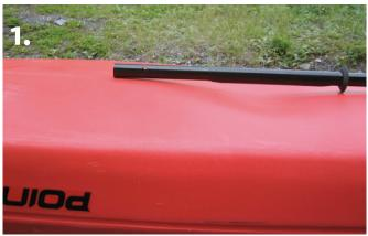
As Polyethylene has a built in "memory" in the molecules it is actually striving to get back into shape and just needs a little bit of heat and love to get there.
